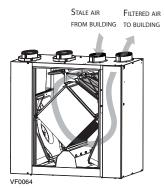
The G3000E ECM uses a unique defrosting method. No negative pressure is created by air exhausted to the outdoors, as the air is recirculated into the house, helping to prevent any backdraft.
